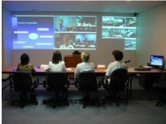
Figure 1: A typical Access Grid set up with 3 projectors, front and ceiling cameras, microphones and the control machine on the right hand side
